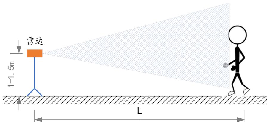
Figure 4-1 Horizontal installation method detection diagram
