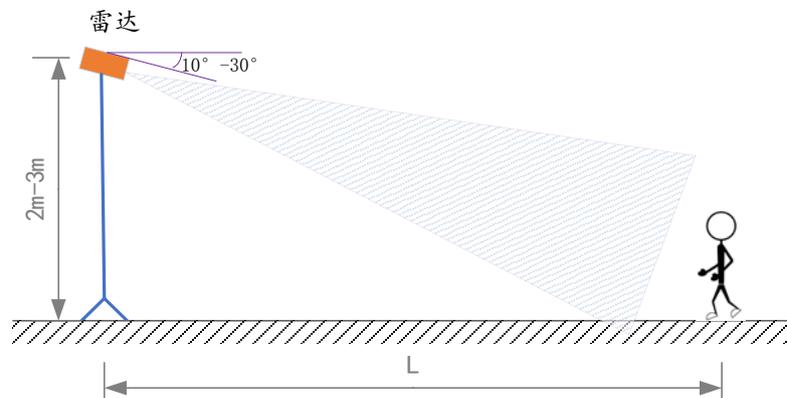
Figure 4-2 Detecting diagram of oblique installation
