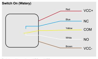
Red wire and brown wire ---- VCC+ and VCC-Yellow wire ---- Relay common pin Blue wire ---- Relay normal closed pin White wire ---- Relay normal open pin
