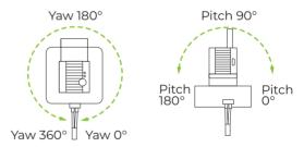
After assembly, when all screws are properly tightened, you should feel the physical limits of the pitch (0°–180°) and yaw (0°–360°) axes. When programming, we recommand add protective code/logic to limit yaw to 9°–340° and pitch to 9°–175° in order to prevent motor damage.
