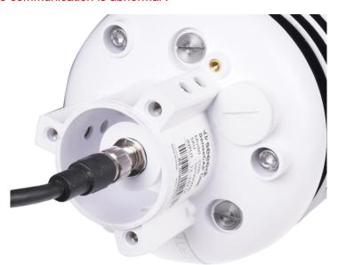
When using the device with a heating function, a separate 24V (24V@1A is recommended) power supply is required. Gray wire #5 is connected to the negative of the power supply, and pink wire #6 is connected
