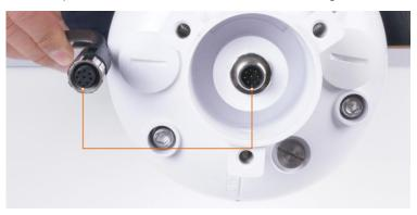
Plugin the cable and tighten it clockwise
