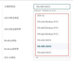
2. Modify the Modbus address: write the address in the Modbus address, and then click "Write to Device".
