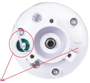
Note: The white caps should be screwed down after commissioning, to prevent water from the device!
