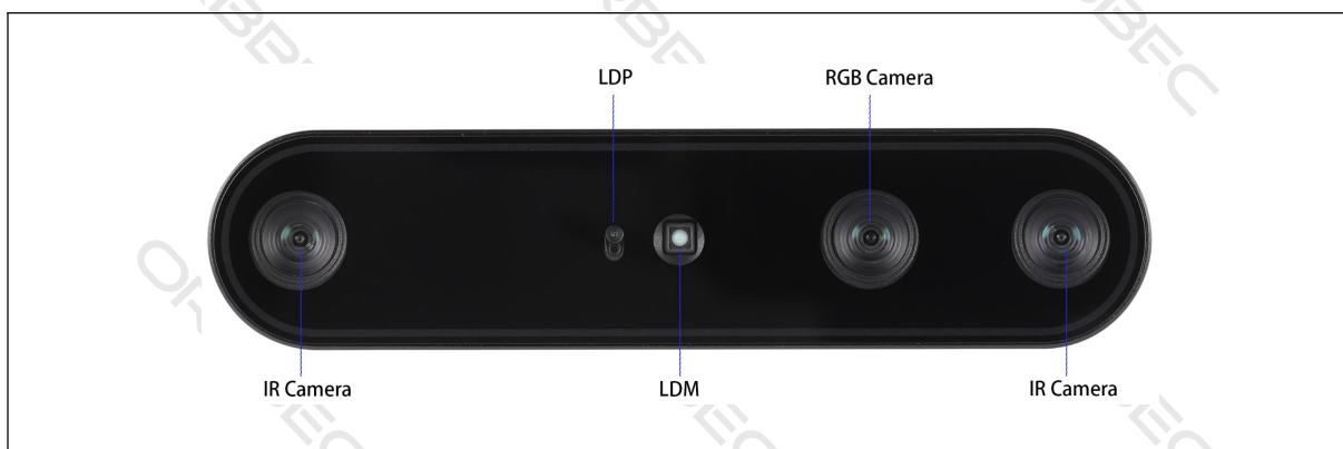
Figure 3-2-3 Gemini 2 L Product Diagram
