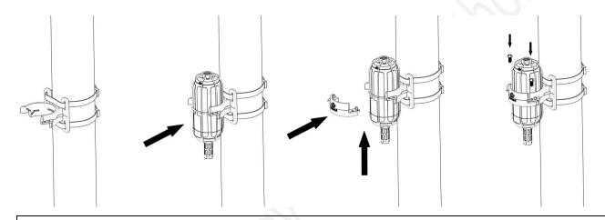
**Note:** Do not insert the Sensor Node into the bracket from the top, or it will not fasten the onto the bracket securely.
