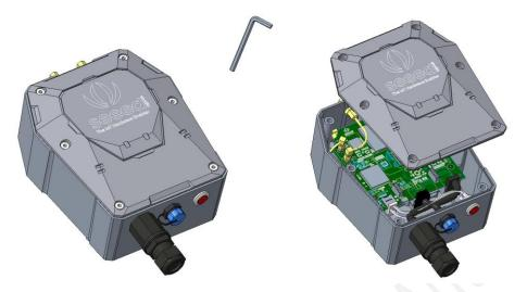
Swipe downward to open the SIM card socket, insert the Micro SIM card and swipe upward to lock the SIM card socket. Make sure it is installed correctly and close the lid with the screws.
