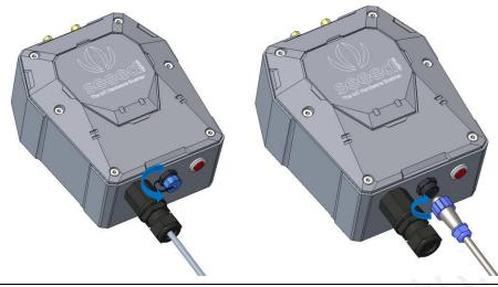
**Notice:** Make sure all antennas are correctly installed before powering on the gateway. Please note the device should be POWERED OFF when installing the antenna, or the antenna circuits might be damaged.
