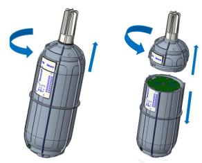
5) After opening the device, turn the switch to "ON", and the LED on the lower right corner will flash, indicating that the power is on. Wait for about 10 seconds, then the LED will flash quickly for 2 seconds, indicating that the device is connected to the network.
