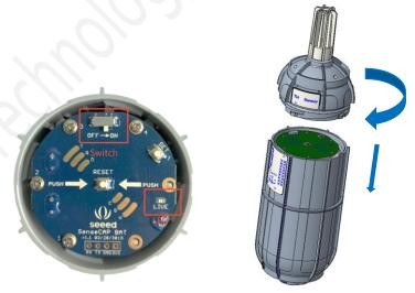
3) After the device is connected to the network, connect the Sensor Probe back with the Sensor Node Controller by turning it clockwise. Please note that the labels on both parts should be aligned as shown in the image below, otherwise the two parts will not be attached to function properly and data will not be uploaded.
