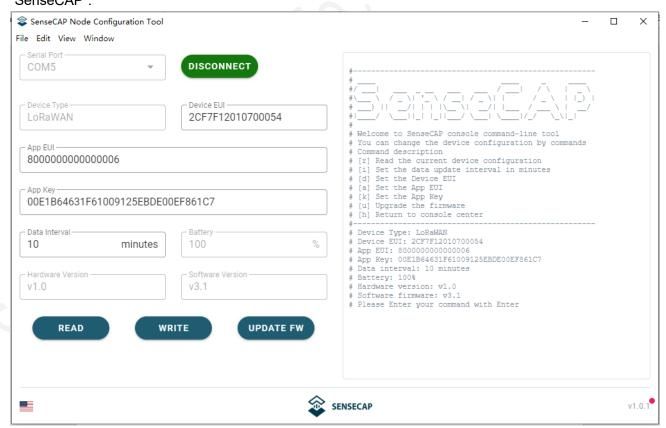
(4) ①Device EUI (16 bit) ②App EUI (16 bit) ③App Key (32 bit) ④Data Interval (Sensor collection cycle)
