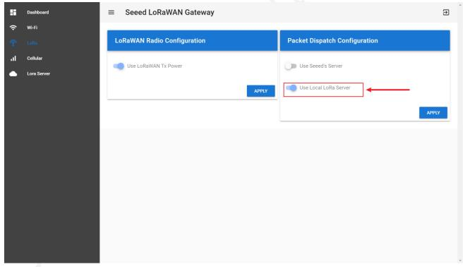
(5) Turn on the "Use LoRa Server" button, and apply. ("LoRa Server" is the name of ChirpStack LoRa Server)
