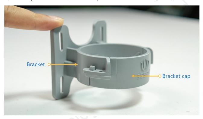
1) To install on a pole, you can use zip ties to fasten the bracket (recommended pole dimension is 50-70mm in diameter). Please refer to the following image for bracket directions.
