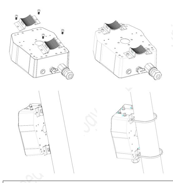
**Note:** If the pole is made of metal, the antenna should be pulled higher than the metallic part of the pole, or the communication signal will have interfered.
