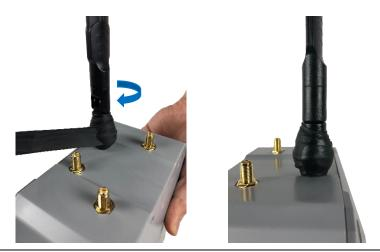
**Note:** The tape must be wound clockwise because the antenna is fastened clockwise. Otherwise, the antenna may loosen.
