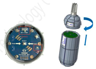
6) After the device is connected to the network, connect the Sensor Probe back with the Sensor Node Controller by turning it clockwise. Please note that the labels on both parts should be aligned as shown in the image below, otherwise the two parts will not be attached to function properly and data will not be uploaded.
