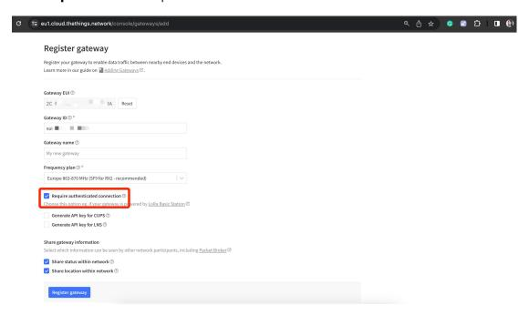
This will only allow a gateway to connect if it uses a TLS enabled Basic Station or MQTT connection.
