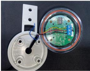
2. Turn the DIP Switches  $\bf 1$  of the rain sensor S1 base to the ON, turn the switch  $\bf 2$  to the OFF , and turn the  $\bf 3$  and  $\bf 4$  to the OFF;
