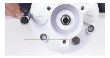
Plugin the cable and tighten it clockwise
