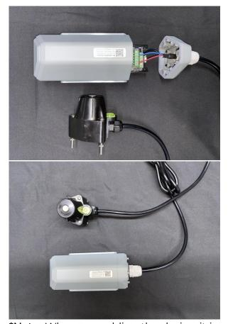
\*Note: When assembling the device, it is necessary to install the waterproof pad of the Data Logger and the adapter box, and tighten the screw cap and screw, otherwise the waterproof effect of the device may be affected!
