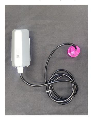
\*Note: When assembling the device, it is necessary to install the waterproof pad of the Data Logger and the adapter box, and tighten the screw cap and screw, otherwise the waterproof effect of the device may be affected!
