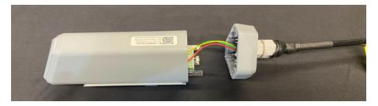
3. **Tighten the screws and screw caps to check the waterproofing**. If the wire diameter is too thin, add waterproof tape for winding.
