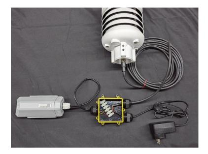
Tighten the screws and screw caps to check the waterproofing. If the wire diameter is too thin, add waterproof tape for winding.
