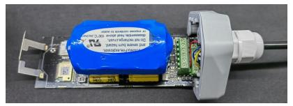
3. **Tighten the screws and screw caps to check the waterproofing**. If the wire diameter is too thin, add waterproof tape for winding.
