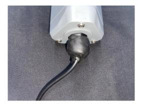
3.9.3 Connect to the Rain Gauge Sensor
