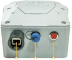
Ethernet Port · Power Connector · LED
