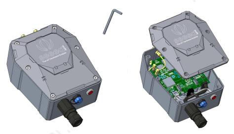
Swipe downward to open the SIM card socket, insert the Micro SIM card and swipe upward to lock the SIM card socket. Make sure it is installed correctly and close the lid with the screws.
