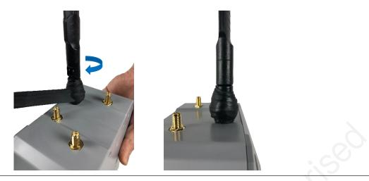
**Note:** The tape must be wound clockwise because the antenna is fastened clockwise. Otherwise, the antenna may loosen.
