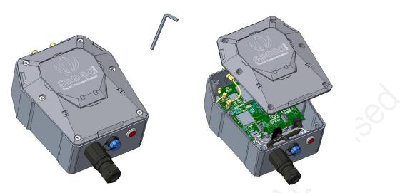
Swipe downward to open the SIM card socket, insert the Micro SIM card and swipe upward to lock the SIM card socket. Make sure it is installed correctly and close the lid with the screws.
