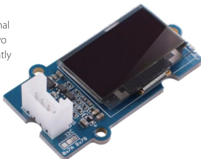
When we allow the current flow in circuit electrons cross border between these two materials and release surplus energy, giving off a quick flash of light. All those flashes produce the dull, continuous glow. A simple OLED is made up of six different layers.
