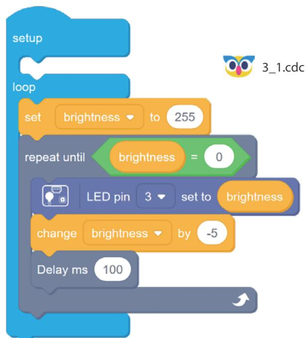
Remember, that LED module still needs to be connected to Pin 3 with Grove cable, since Pin 3 can use PWM and Pin 4 cannot.
