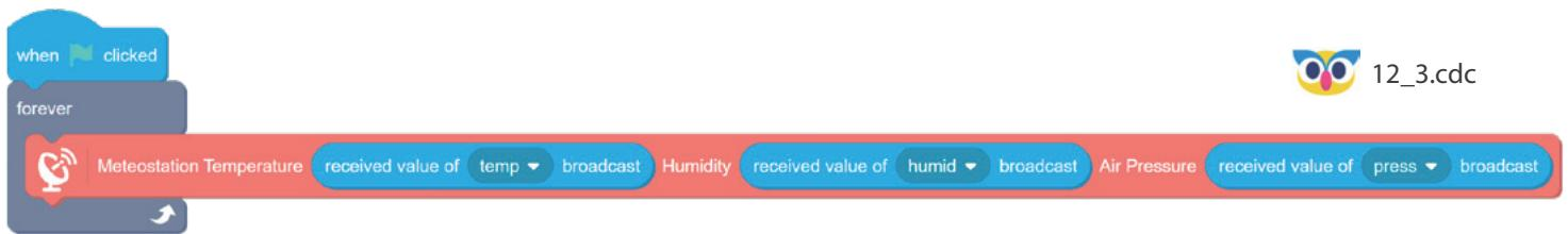
Connect to Arduino in Device mode as you usually do when use Serial monitor or Plotter. Then go to stage mode, press the flag button and click on **Open meteostation window** button in Meteostation category. The data from sensors will be displayed and updated in real time on meteostation interface!
