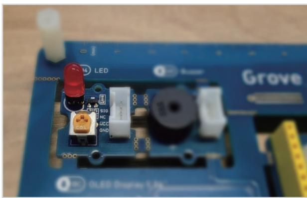
Not really. The microchip inside of our board did exactly what you instructed it to do - it closed the circuit allowing the electrons to flow and then opened it stopping the flow of electrons. It is just it happened way too fast for your eyes to see the difference. Let's add delay block, which you can find in Control category, to slow things down a bit. And here we have it! Our first blinking LED!
