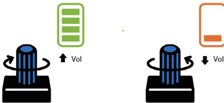
To use scientific terminology, potentiometer can be used as rheostat (variable resistor) or as a voltage divider. If you remember from the previous lessons, changing voltage in the circuit is exactly what we did programmatically to dim the LED. Only in this lesson instead of outputting different voltages with our Grove Beginner Kit, we are going to measure and display the input voltage and see its number representation changes as we turn the handle.
