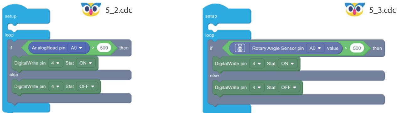
We will still use the dedicated blocks for modules, just for the sake of aesthetics and convenience. The input voltage range of ADC converter in our board is from 0 to 5V - when it receives 0V, it will output value 0. When it receives 5V, it outputs value 1023. So, 500 should be about 2.5V or half of full rotation of the handle. Try out and see the result!
