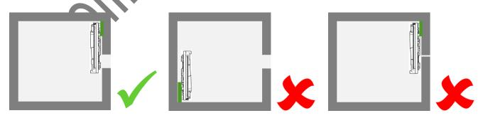
To enable fastest response times the inner open volume of the device should be designed as small as possible. It is recommended to mount SCD30 such that the bottom side of the sensor faces the host PCB, however SCD30 can also be mounted upside down.
