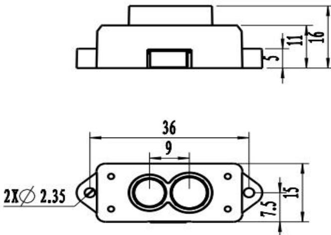
Fig. 6 TF\_mini left module size drawing (unit: mm)
