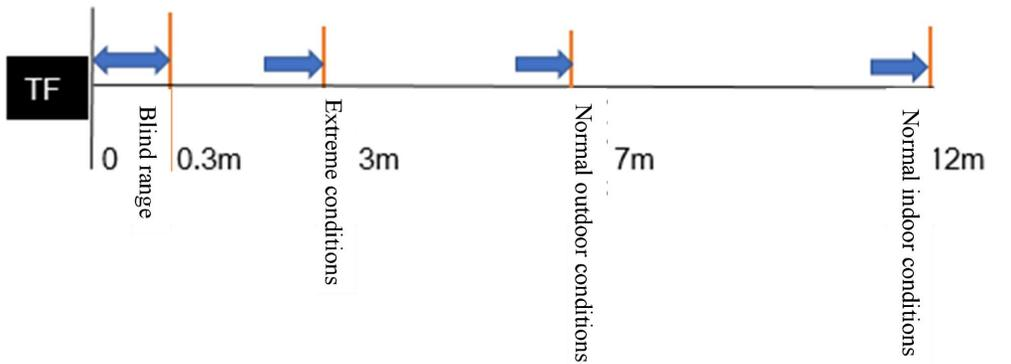
Fig. 2 Measurement range schematic diagram
