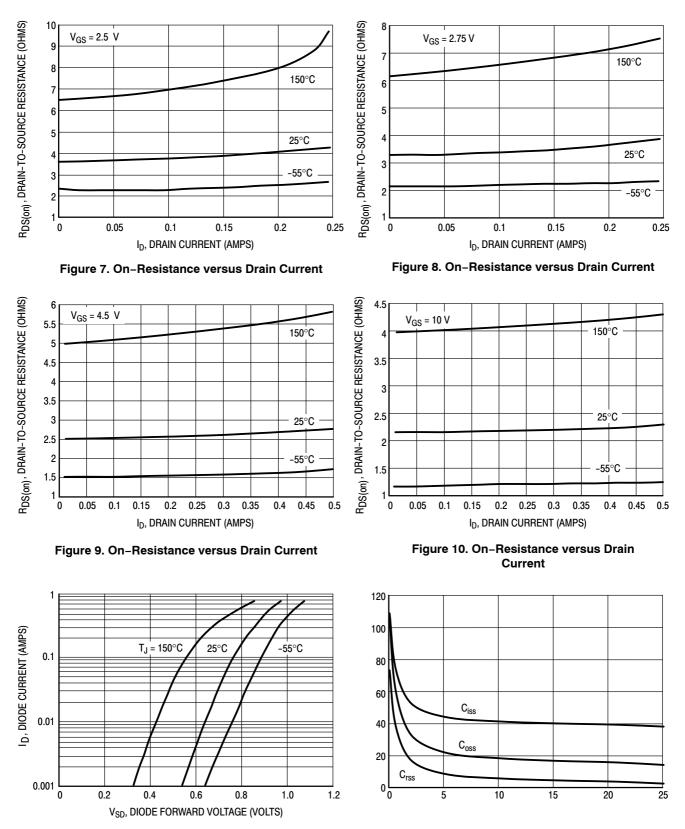
Figure 11. Body Diode Forward Voltage
