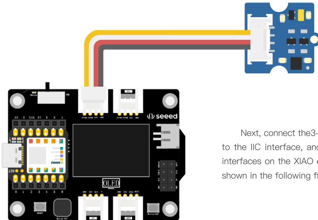
Next, connect the 3-axis accelerometer to the IIC interface, and there are two IIC interfaces on the XIAO expansion board as shown in the following figure.
