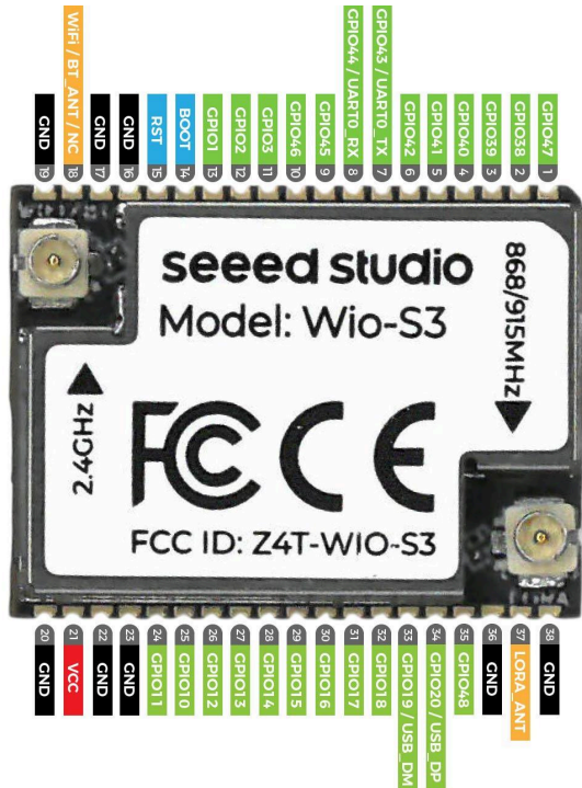
Fig. 2: Wio-S3 Pin arrangement
