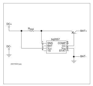
Figure 5. High-Side Current Sensing
