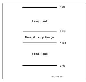
Figure 10. bq2057 TS Input Thresholds
