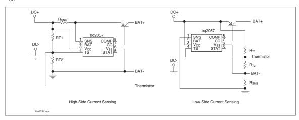
**Figure 9. Temperature Sensing Circuits**
