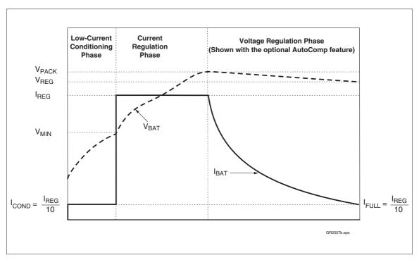
Figure 4. bq2057 Typical Charge Algorithm
