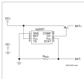
Figure 6. Low-Side Current Sensing
