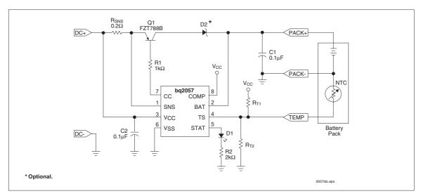
Figure 3. Low-Dropout Single- or Dual-Cell Li-lon Charger
